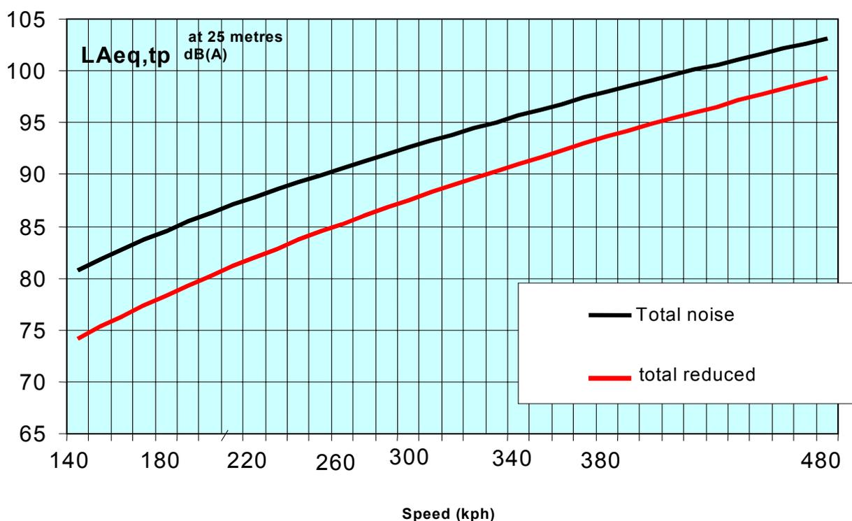
with wheel and track dampers, and bogie shrouds on motor coaches), where 7 dB(A) reduction are achieved on rolling noise and 3 dB(A) reductions on aerodynamic noise.
