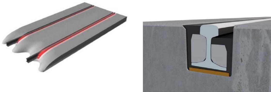
**Graph 17. Example of an embedded rail support in a concrete slab (right: Edilon Sedra; source: Wikipedia).**
