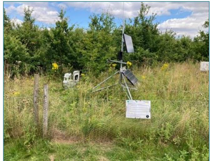
(Figure 1: Autonomous biodiversity monitoring station on the lineside (left), Small mammal camera trap (right), © Network Rail)
