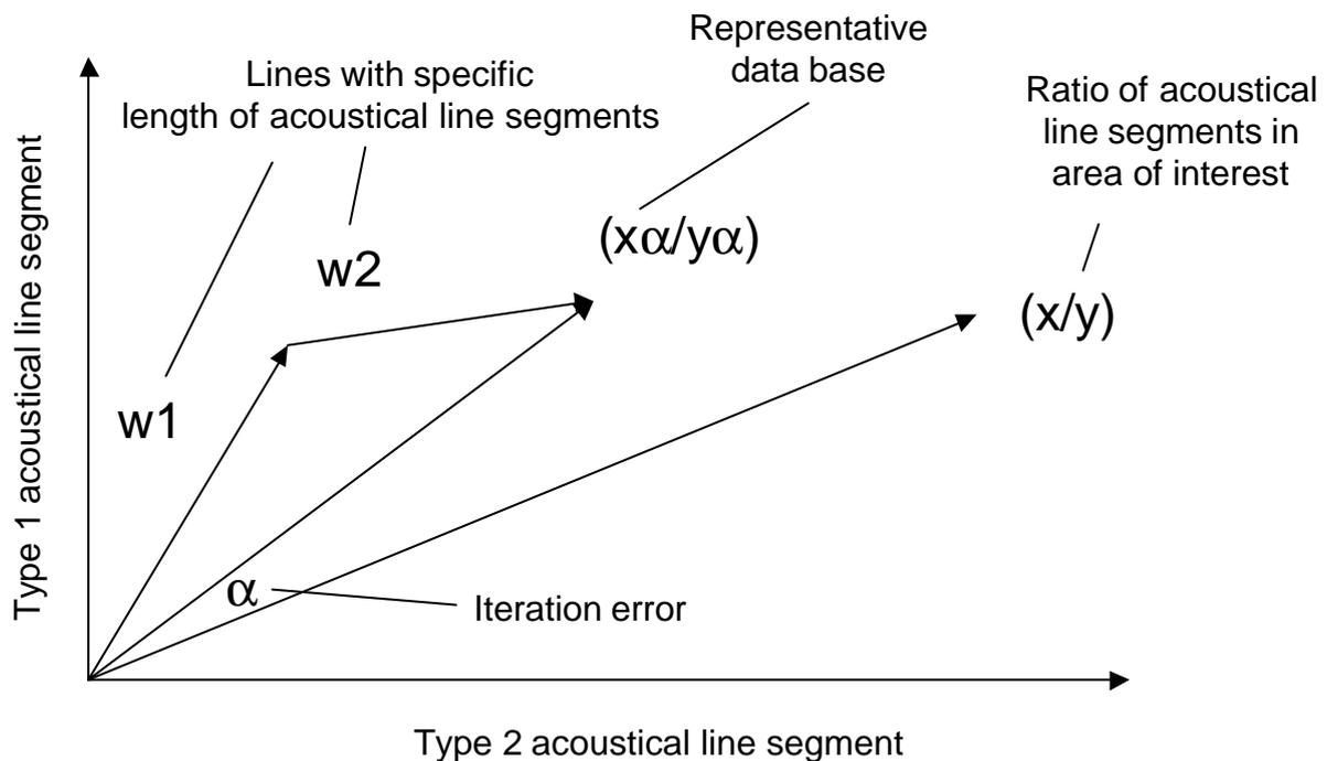
Figure 10: Illustration of iteration process to find representative data base.
