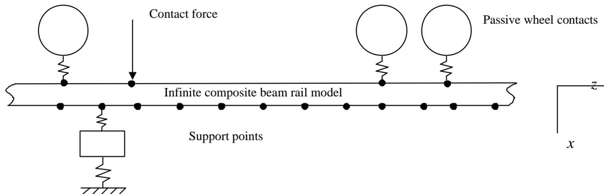
**Figure 21.** Diagram of the new track model, ‘cobra’.
