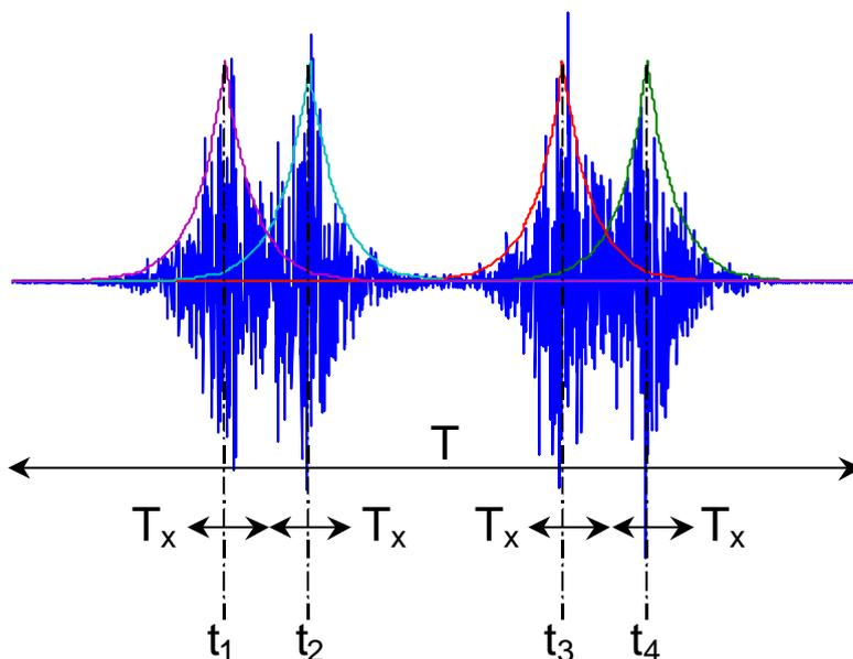
Figure 16: Vertical acceleration measurement during four wheel passages.
