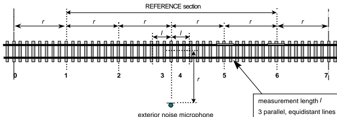
**Figure 29: ISO procedure, with extended sections 0 and 7.**
