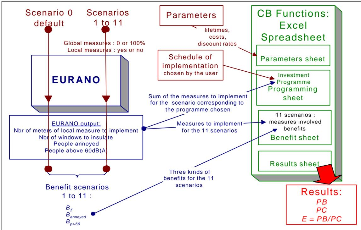
Figure 6 Data flow between EURANO and the "CB Functions" Spreadsheet.
