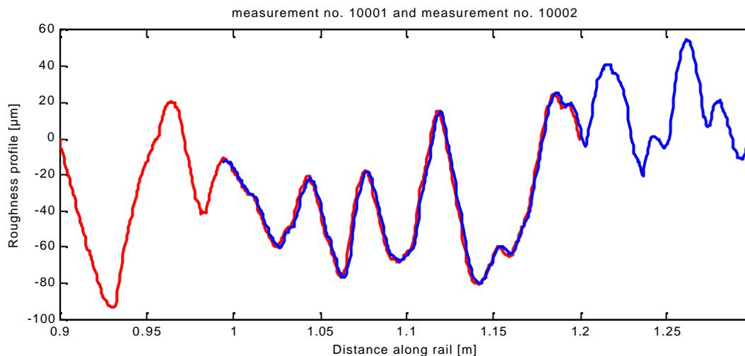
**Figure 32: Result of automatic least squares fitting after manual shifting.**
