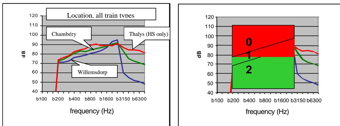
**Figure 41: Example of Track Transfer Function Classification**
