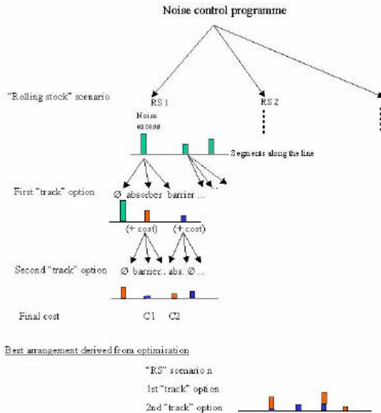
Figure 13: Illustration of the branch and bound method.
