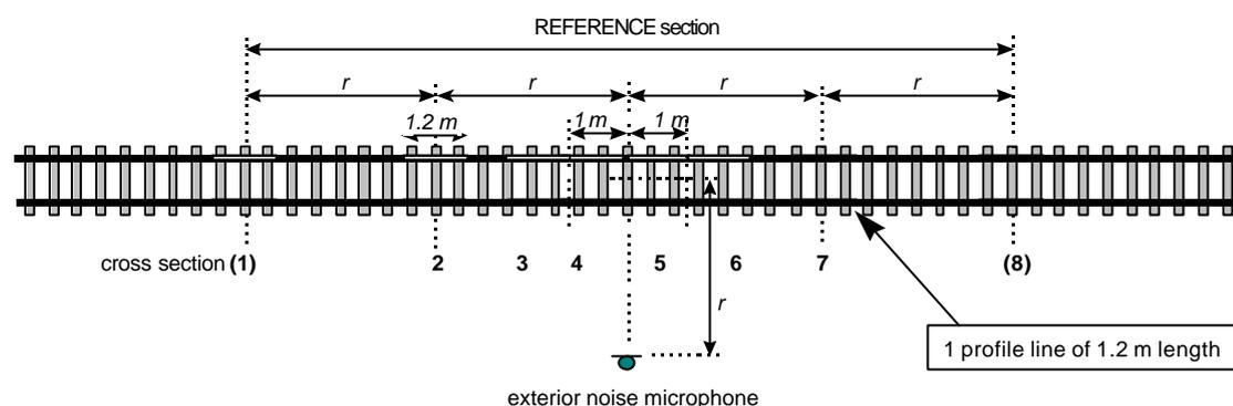
**Figure 25: Required procedure for rail roughness measurement with instruments of 1.2 m length**
