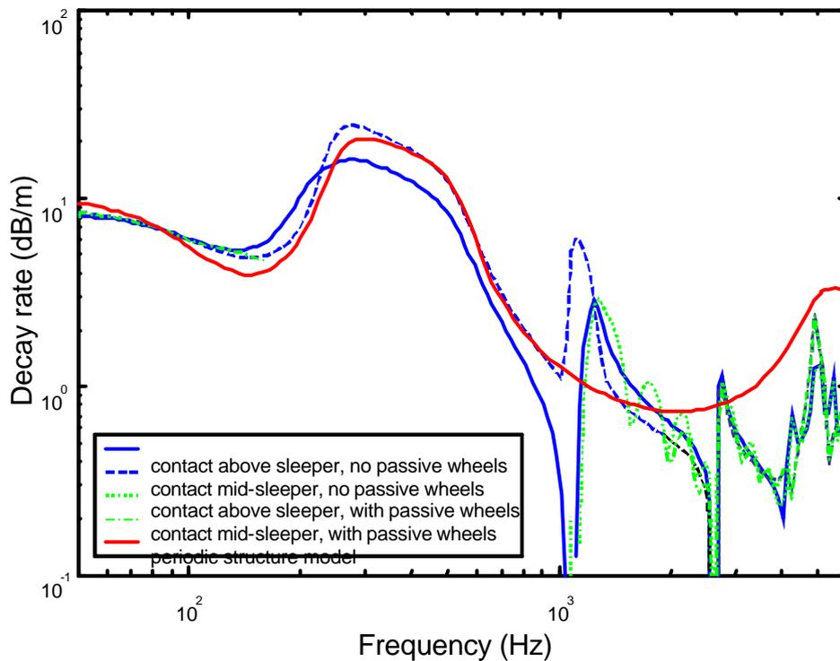
**Figure 23.** Vertical decay rates calculated using the periodic structure model and the new model.
