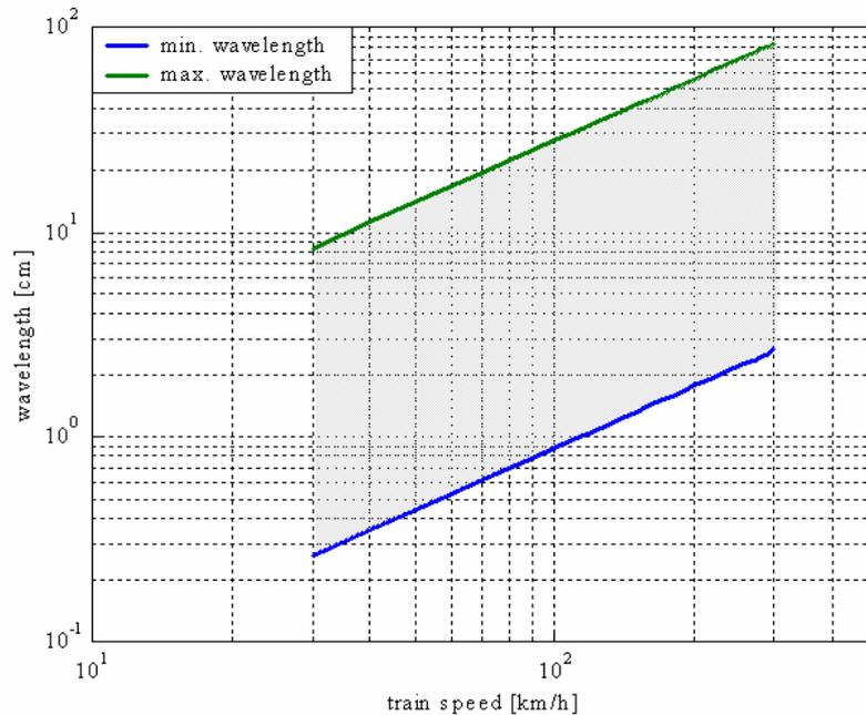
Figure 19: Maximum wavelength range that can be covered by the indirect roughness method as a function of the pass-by speed.
