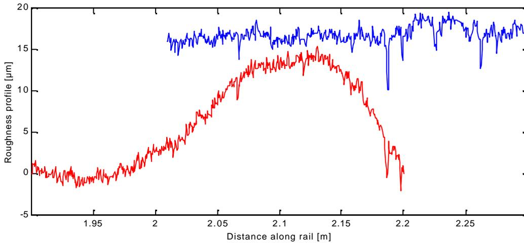
**Figure 35: Badly aligned data due to uncalibrated instrument.**
