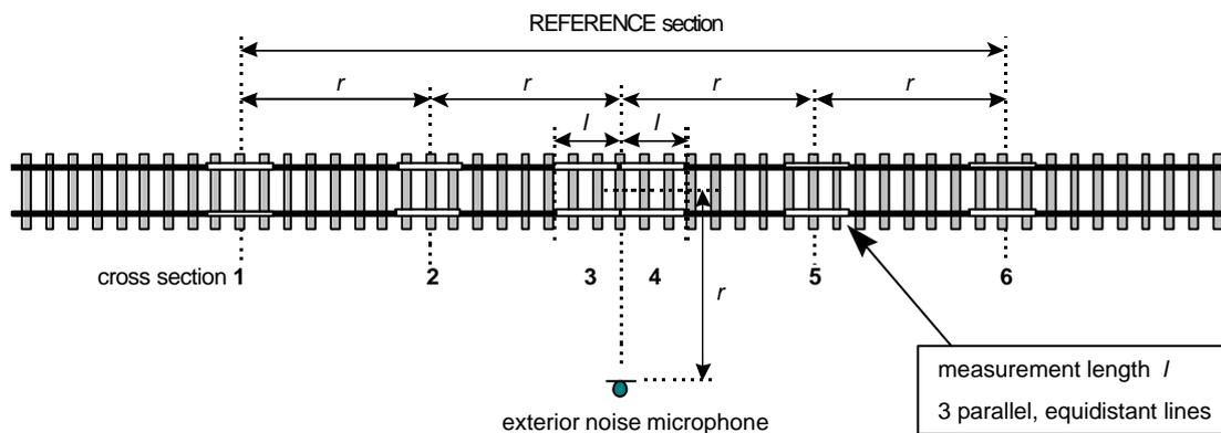
**Figure 27: Measurement map for rail roughness**
