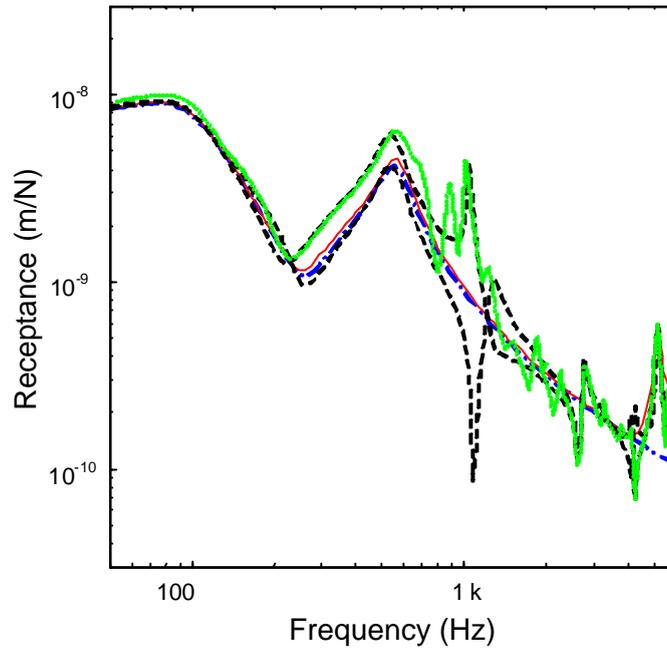
**Figure 22.** Direct vertical receptance at the contact (- - - Timoshenko beam model; — periodic structure model; - - - new model with contact over sleeper and midway between sleepers; ···· new model with one carriage of passive wheels, contact at mid-span position).
