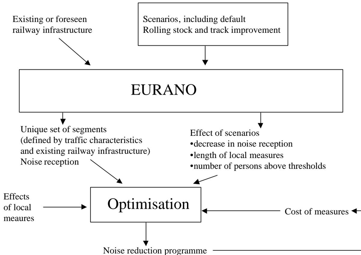
Figure 14: Process diagram showing interaction of optimisation with Eurano.
