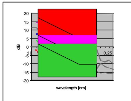
**Figure 39: Example of Rail Roughness Classification**
