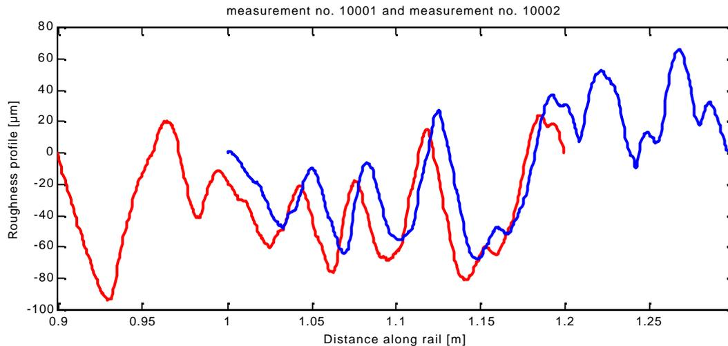
**Figure 31: Fitting procedure. At start, data is displayed assuming exactly 20 cm overlap.**
