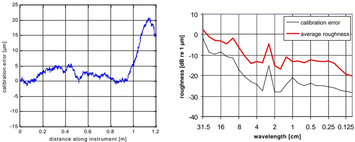
**Figure 36: Left: estimated calibration error or error profile. Right: spectrum of 4 concatenated error profiles.**
