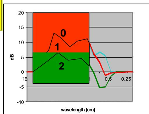
Figure 38: Example of Wheel Roughness Classification
