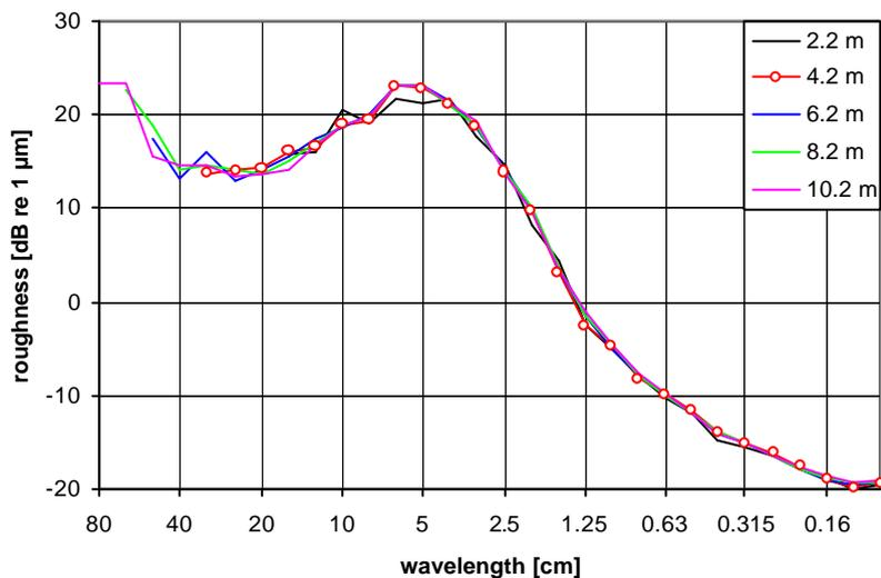
**Figure 33: Roughness spectra for stepwise extending the concatenation length from 2.2 m to 10.2 m.**
