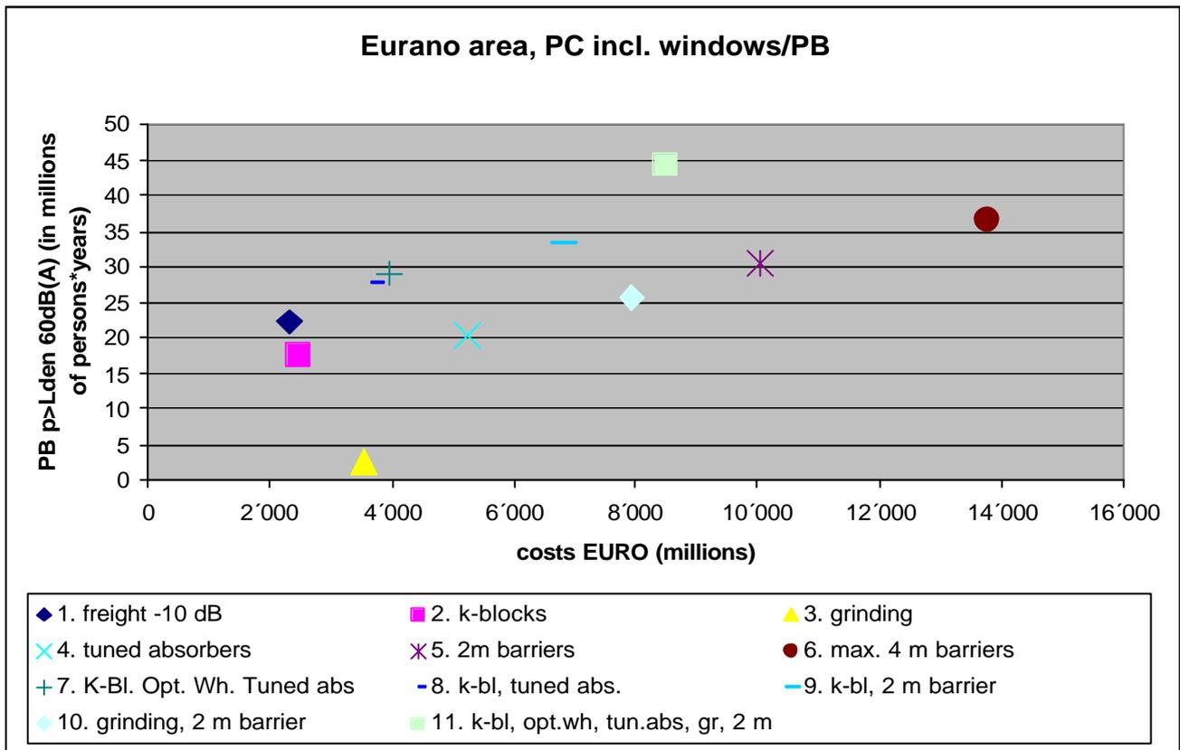
Figure 8: Discounted costs and effectiveness for Eurano area using short term approach, including cost of insulated windows
