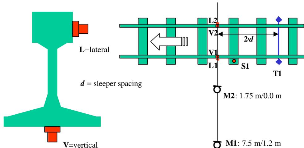
**Figure 24: Position of transducers on the track.**
