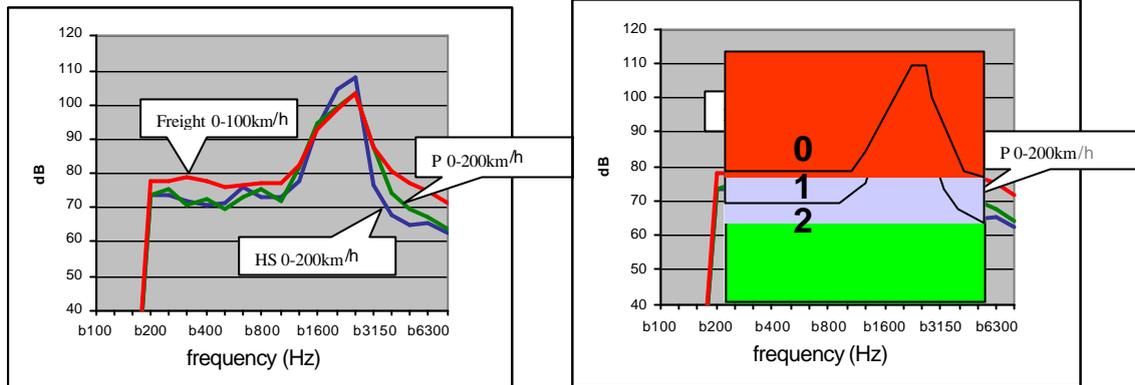
**Figure 40: Example of Vehicle Transfer Function Classification**
