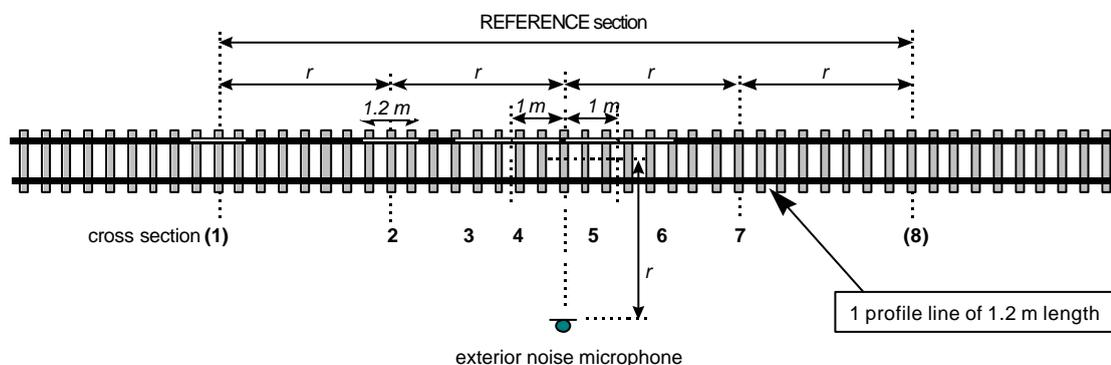
**Figure 37: New proposal for rail roughness measurement procedure for instruments of 1.2 m length**
