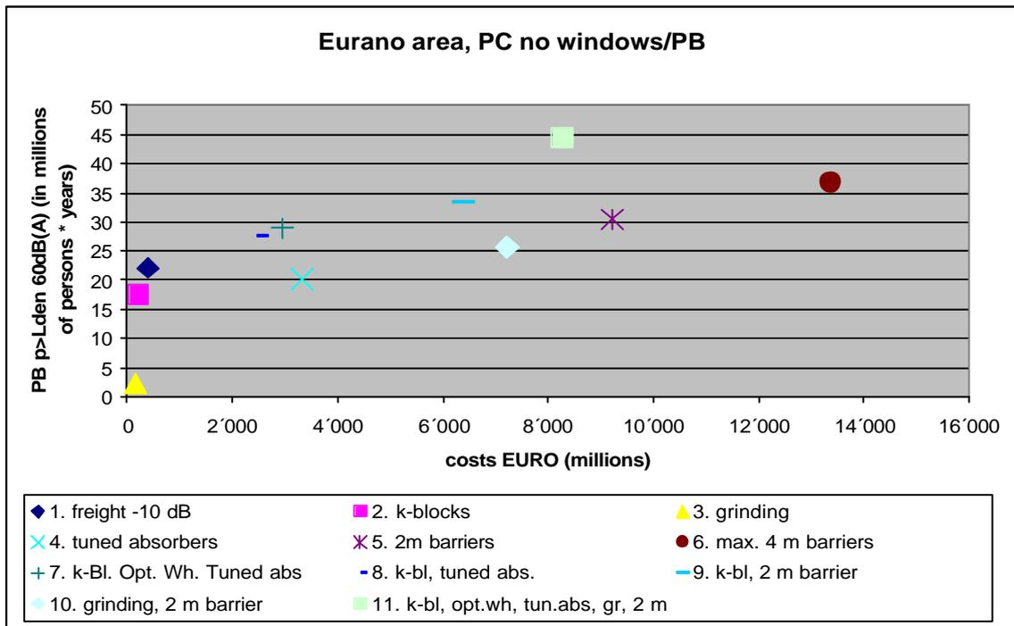
Figure 7: Discounted costs and effectiveness for Eurano area using short term approach, excluding cost of insulated windows
