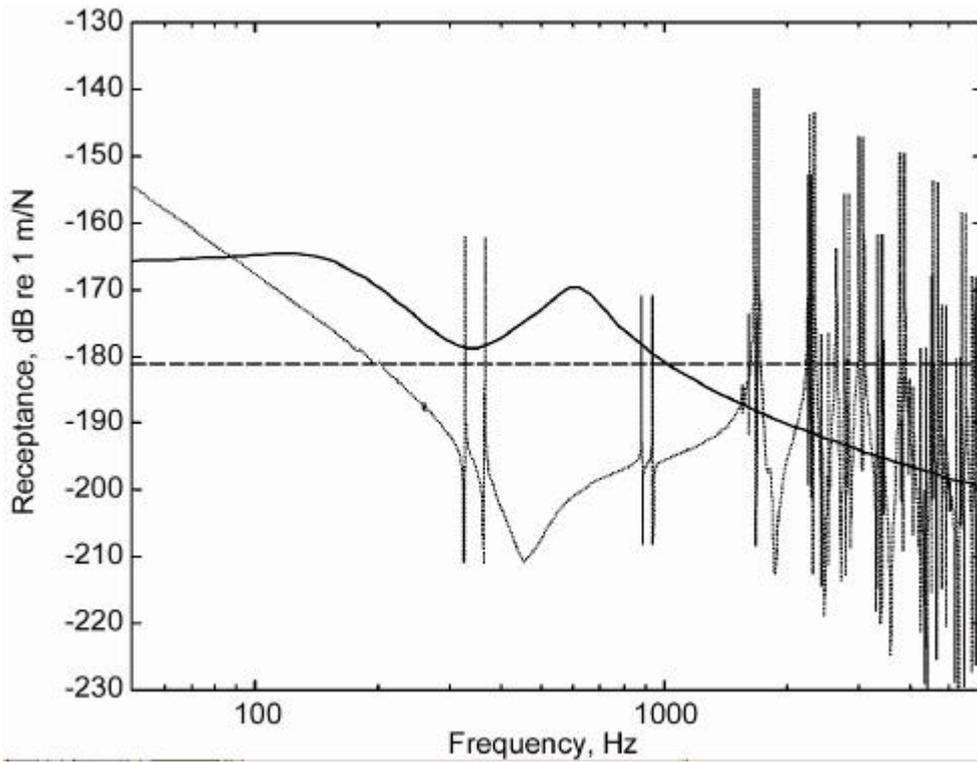
Figure 17: Vertical receptances for reference situation: — rail, - - - contact stiffness and ..... wheel.
