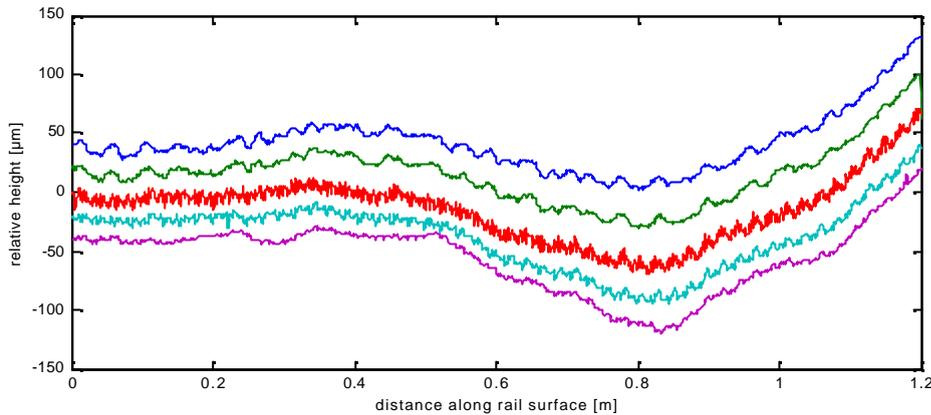
**Figure 28: Oosterbeek track.: 5 parallel profile lines, lateral offset on the railhead –10, -5, 0, 5 and 10 mm, respectively.**
