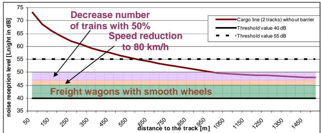
Figure 32: To reduce noise reception levels to 40 dB requires substantially operational measures. Even for large distance to the track these measures will not reduce enough.
