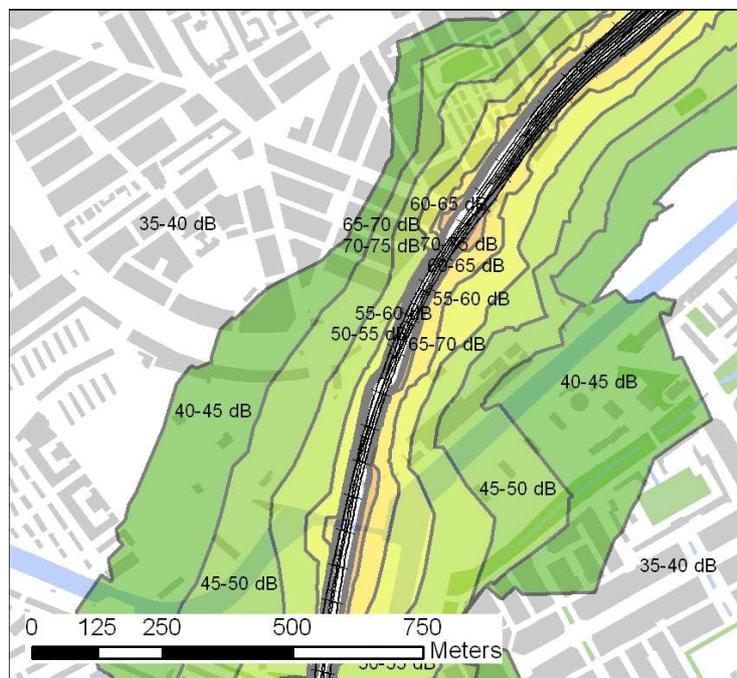
Figure 18: Example of distance of railway noise levels for present situation ( $L_{night}$ ).
