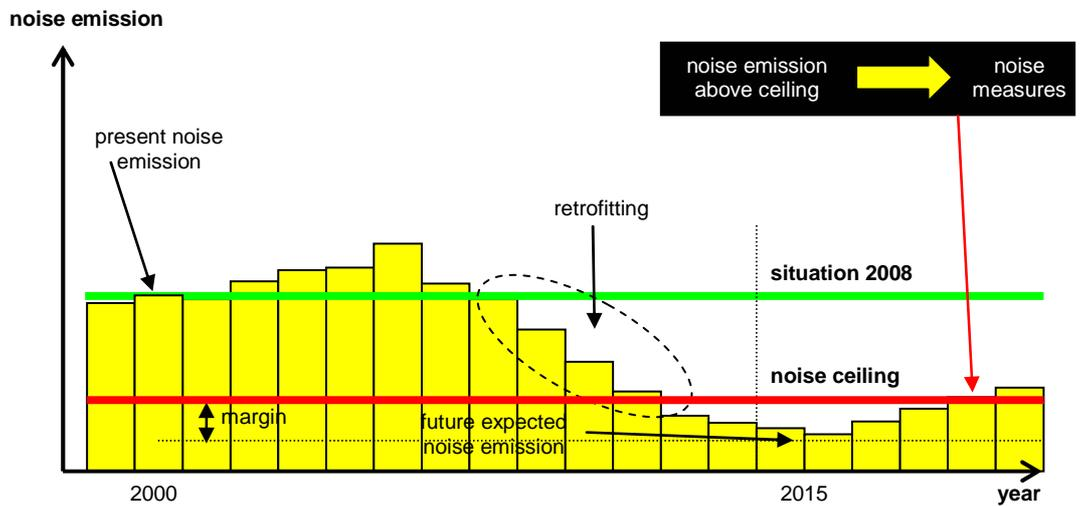
Figure 22: Graphical presentation of the ‘Swiss system’ of noise emission ceilings. The margin is different for different railway lines, based on a traffic prognosis for each line.
