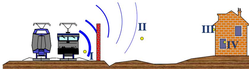
Figure 4: Noise limits are defined at different spots between source and receiver.
