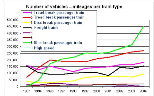
*Still a considerable number of passenger trains with cast-iron blocks (type 1 and 2 ) is running on the Dutch network.*
