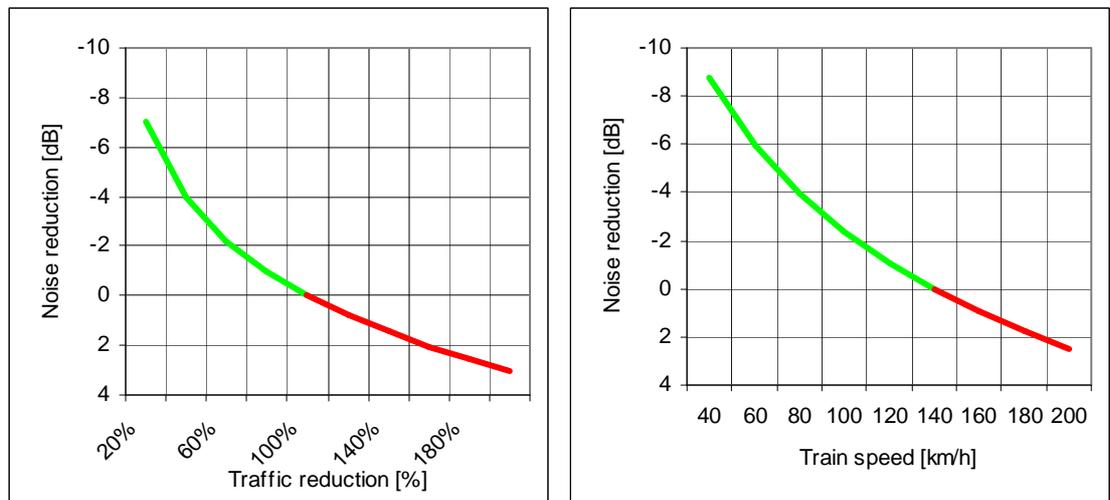
Figure 35: Substantially operational measures like traffic reduction and reduction of train speed do have a relative small impact noise reduction.
