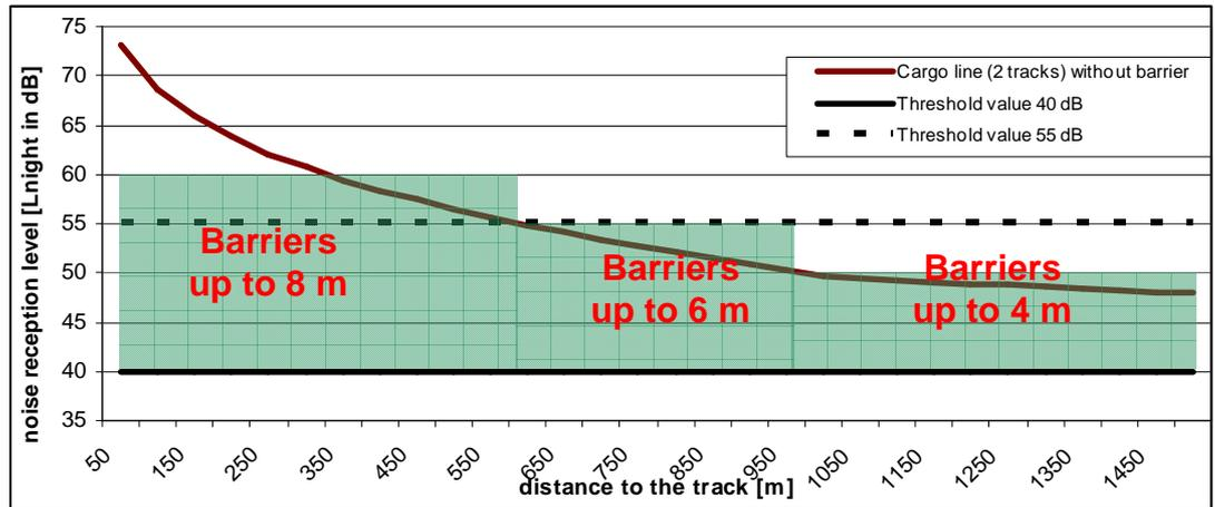
Figure 30: To reduce noise reception levels to 40 dB ( $L_{night}$ ) requires high barriers up to large distance of the track for cargo lines.
