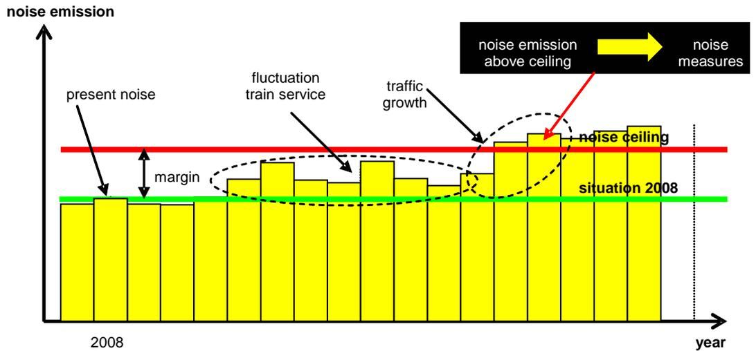
Figure 21: Graphical presentation of the ‘Dutch system’ of noise emission ceilings. The margin is 1.5 dB on the whole network.
