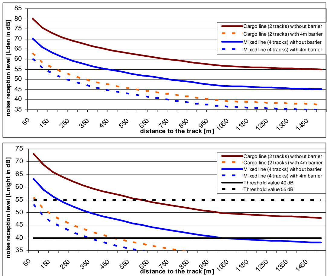
Figure 25: Example of noise reception levels relative to the distance to the track for a cargo line and a mixed passenger/cargo line. Above the  $L_{den}$  value and below the  $L_{night}$  value.
