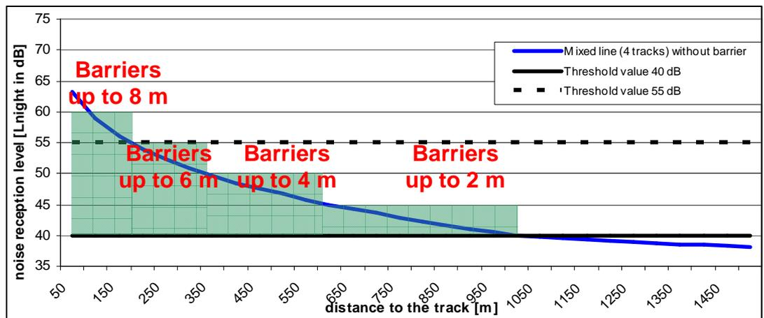
Figure 31: To reduce noise reception levels to 40 dB ( $L_{night}$ ) requires high up to large distance of the track for mixed lines.
