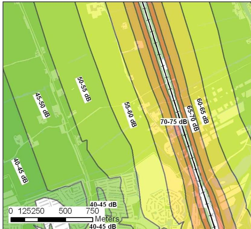
Figure 33: Example of distance of railway noise levels ( $L_{\text{night}}$ ) for present situation. The number of trains used in this figure does not match the number of trains in Figure 25.
