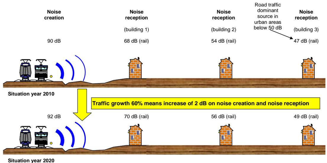
Figure 20: Relative changes in the source lead to corresponding changes at the façade of dwellings. In urban areas reception levels are dominated by road traffic if the levels caused by railways is below 50 dB.
