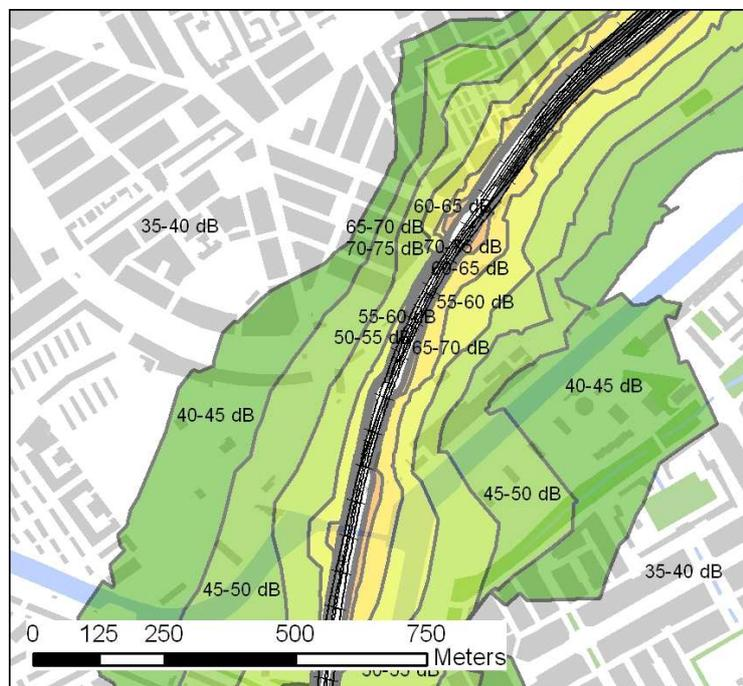
Figure 26: Example of distance of railway noise levels ( $L_{night}$ ) for the present situation. The number of trains used in this figure does not match the number of trains in Figure 25.
