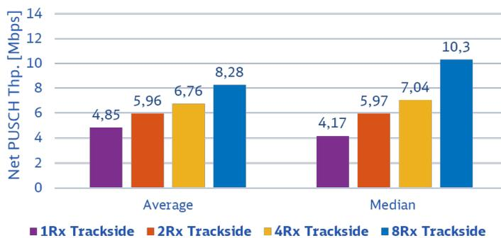
Figure: 3-12: Average and median uplink throughput with Rx diversity for the overall test track
