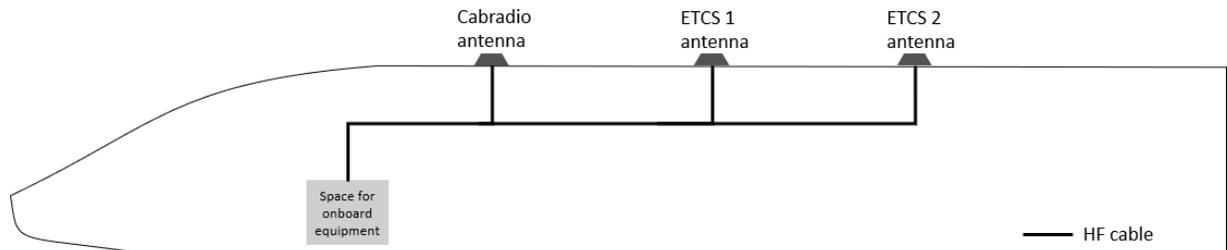
Figure 4-1: GSM-R cab radio and ETCS setup
