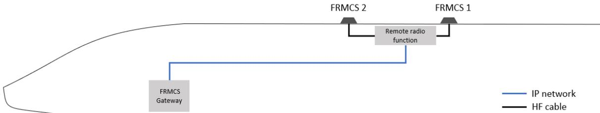
Figure 4-2: FRMCS setup with remote radio function
