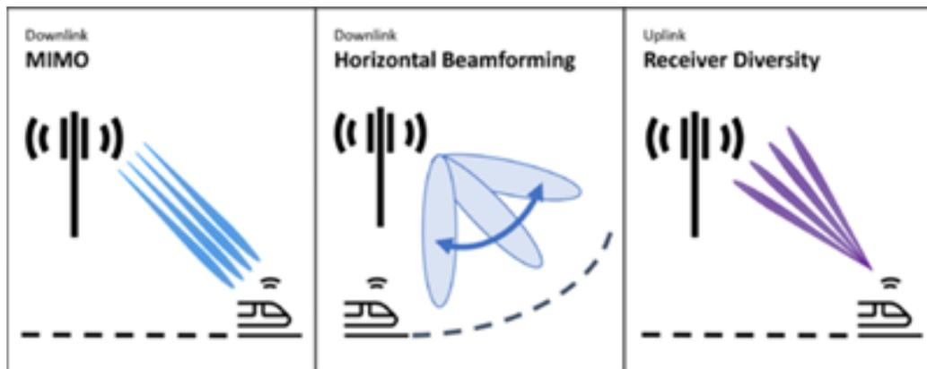
Figure: 3-10: Multi-antenna technologies
