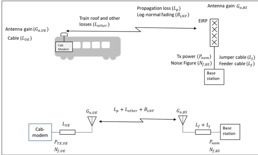
Figure 3-2: System model for FRMCS modem link budgets
