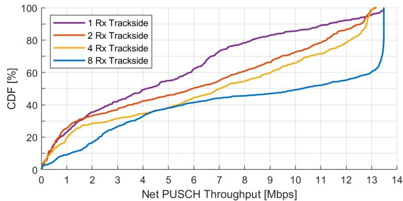
Figure: 3-11: Uplink performance of different trackside antenna configurations with Rx diversity, measured along the overall test track
