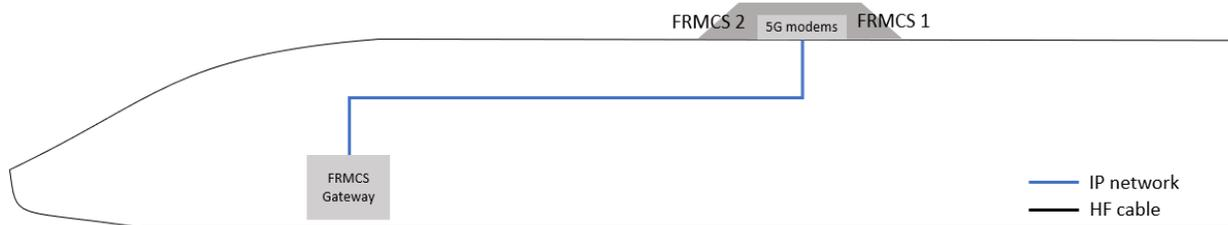
Figure 4-3: FRMCS setup with radio function integrated in antenna
