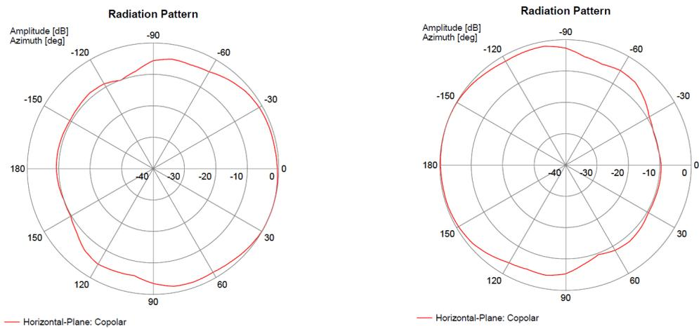
Figure 4-9: Horizontal pattern@1855 MHz (H&S 1399.99.0130; gain ~9 dBi)
