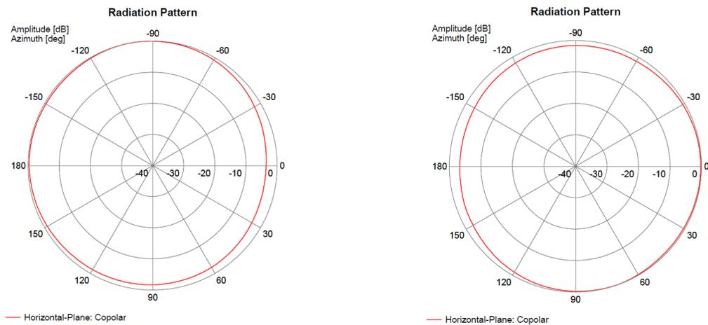
Figure 4-7: Horizontal pattern@ 925 MHz (H&S 1399.99.0130; gain ~7 dBi)
