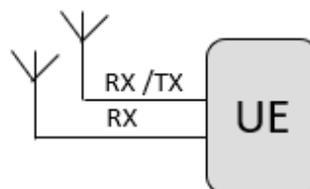
Figure 3-15: UE antenna configuration
