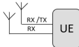
Figure 4-6: UE antenna configuration
