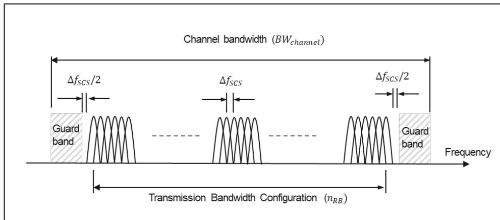
Figure 3-1: Channel bandwidth and transmission bandwidth configuration. From [1, p. 351].
