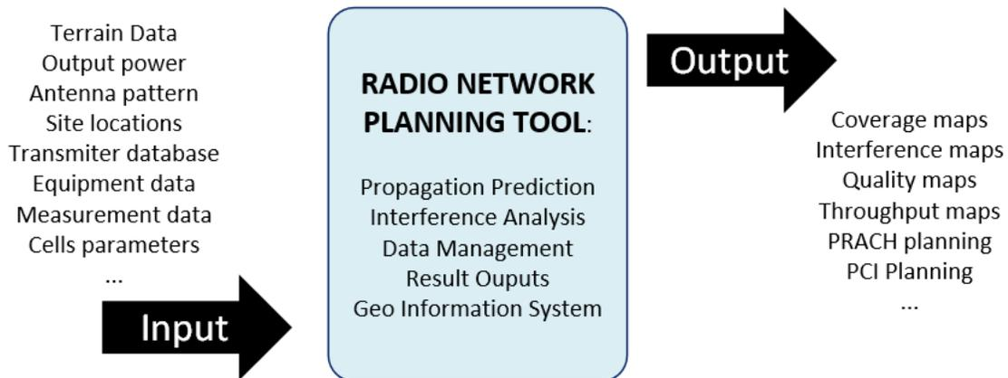
Figure 3-14: Radio network planning process
