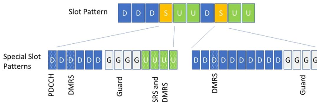
Figure 3-8: TDD pattern for proposed FRMCS pattern DDSUUDSUU (10:4:4, 10:4:0). Subcarrier spacing 30 kHz. DL and UL only slots may contain 1, 2 or 3 DMRS symbols
