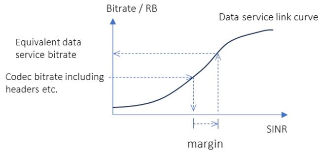
Figure 3-9: Data service link curve
