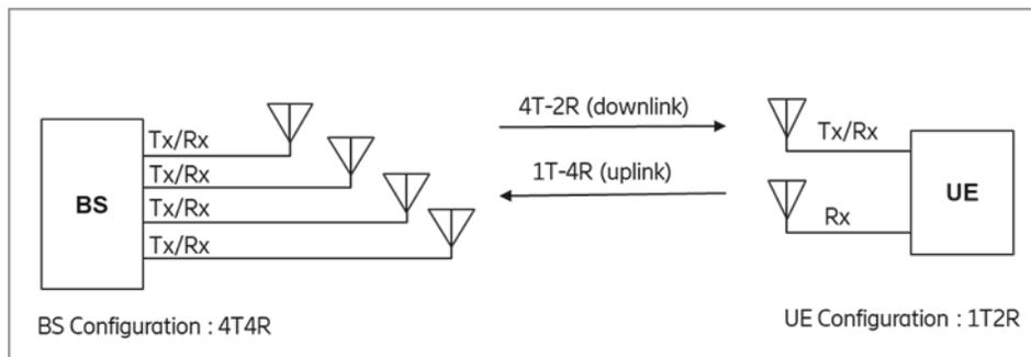
Figure 3-3: Notation for transmission paths and BS and UE antenna configurations
