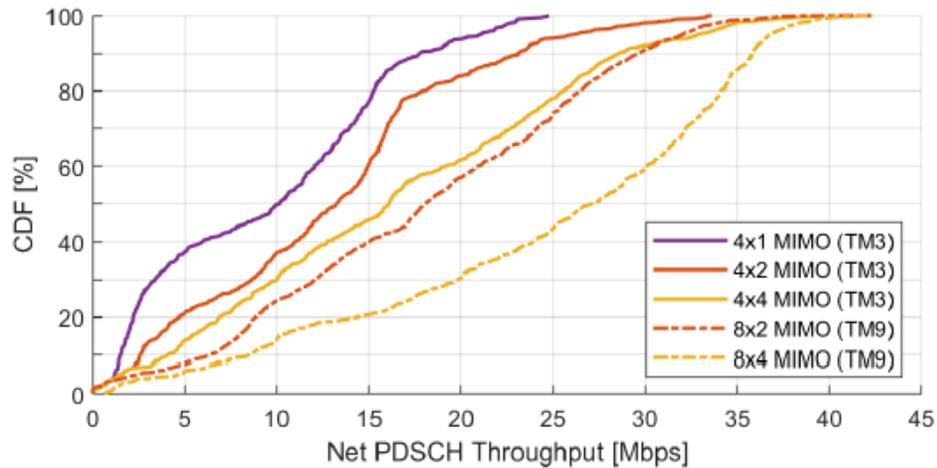
Figure 3-13: Downlink performance of TM3 (MIMO) and TM9 (MIMO & beamforming) configurations, measured along the overall test track
