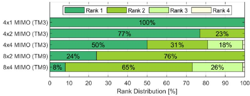
Figure 3-14: Measured rank for the downlink network configurations
