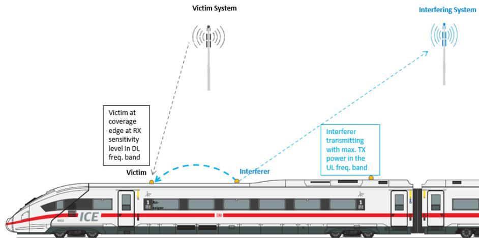
Figure 4-4: Worst case scenario of on-board interference
