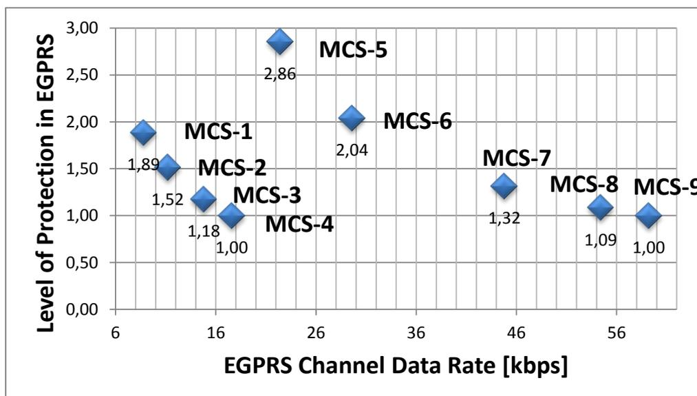
***Figure 2-7 Link between FEC and the resulting Channel Data rate in EGPRS***
