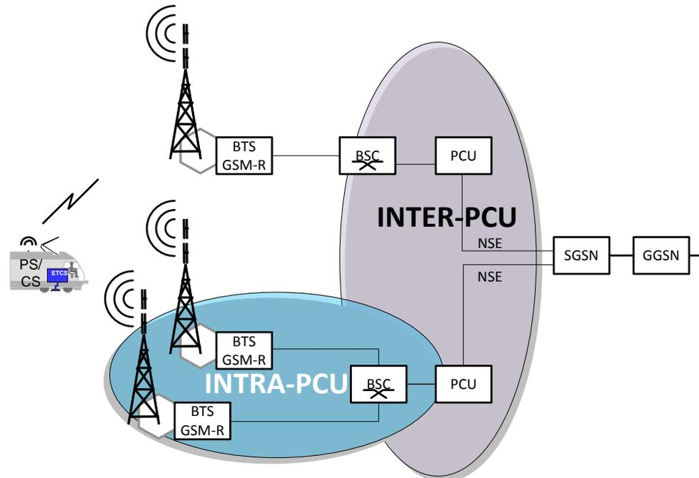
***Figure 4-2 PS-mode - Intra/Inter PCU architecture schematic***
