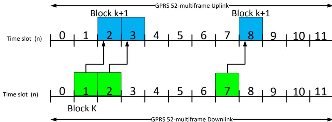
***Figure 3-2 Uplink block allocation principle using USF***
