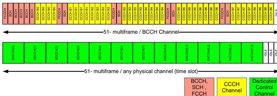
Figure 2-15 Logical Channel sequence non-combined channel setup - Downlink
