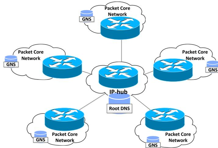
Figure 6-1 PS-mode Roaming - IP-hub
