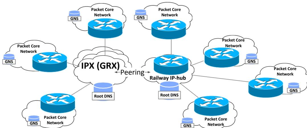
Figure 6-2 IP-hub - IPX peering schematic
