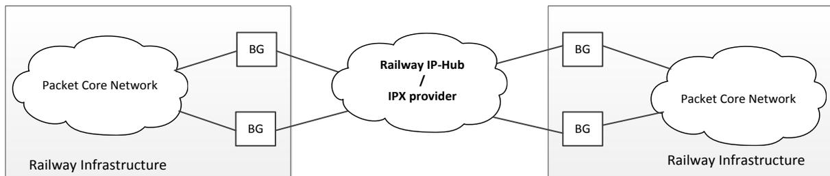
Figure 8-2 Point of Interconnection between IP-hub and the local Packet Core network
