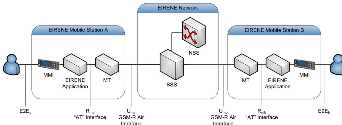
Figure 8: Measurement architecture
