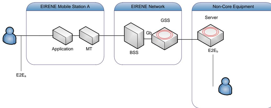
Figure 4: Mobile station user to server measurement architecture
