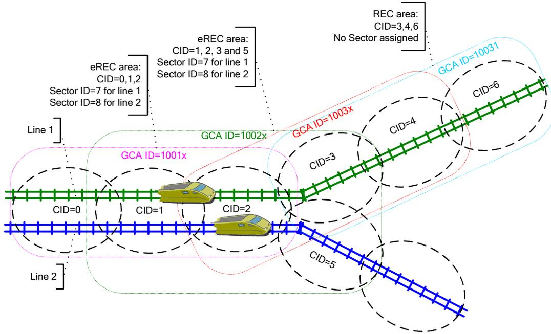
Figure 6 Example of REC and eREC configuration
