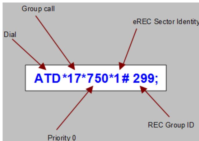
Figure 11 Command for eREC call set up
