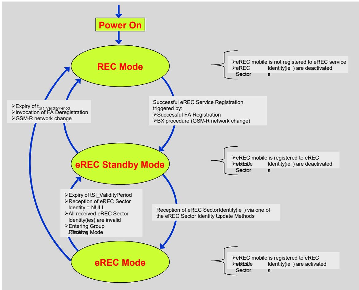
Figure 10 State diagram eREC/REC operation
