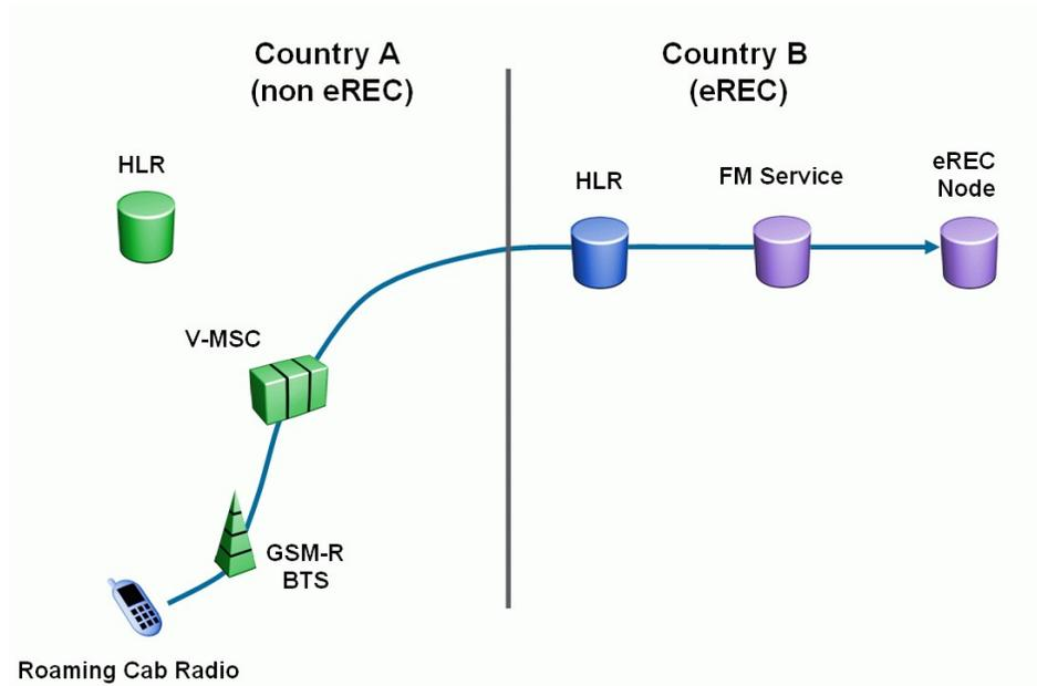
**Figure 8 eREC Service Deregistration of a roaming eREC mobile (cab radio)**
