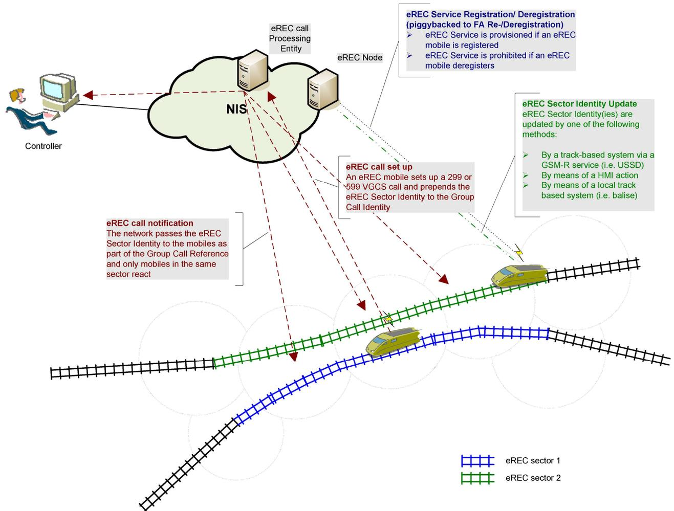
Figure 1 eREC generic system concept
