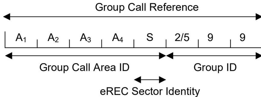
**Figure 2 Structure of the eREC Group Call Reference**
