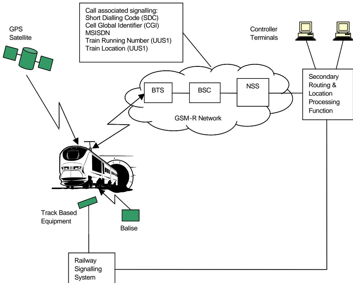
Figure 2-1 Secondary Routing Provided External to NSS
