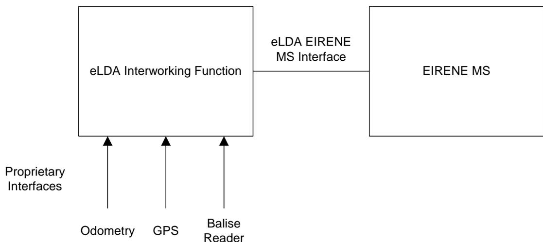
Figure 2-3 Train based architecture
