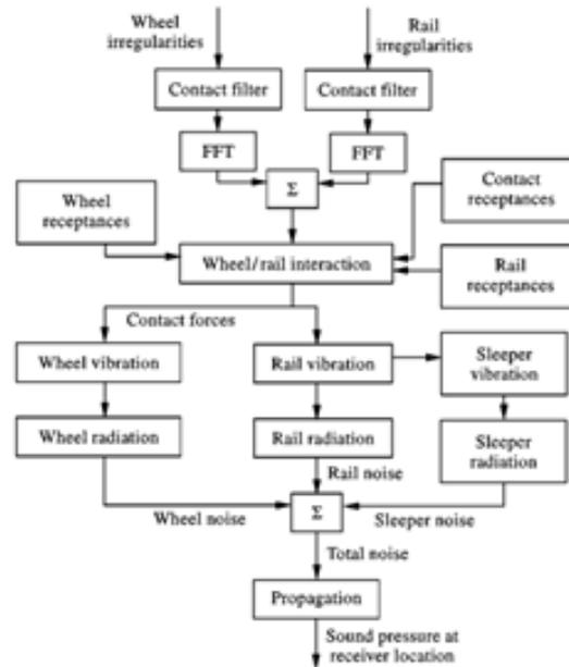
Figure 1 (left): Noise creation mechanism.
