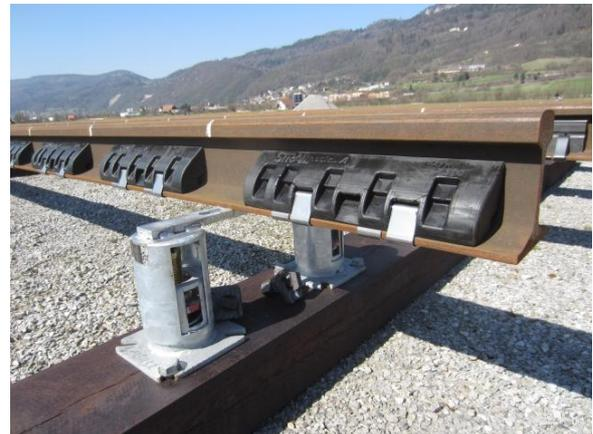
Photographs of the four main damper types. Pictures were taken during the car park tests in Hägendorf (see experience in Switzerland).
