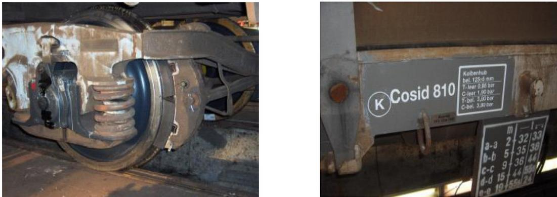
Figure 3.2. Picture of wagon retrofitted with k-blocks. Old wagons such as these are now as silent as modern passenger vehicles.
