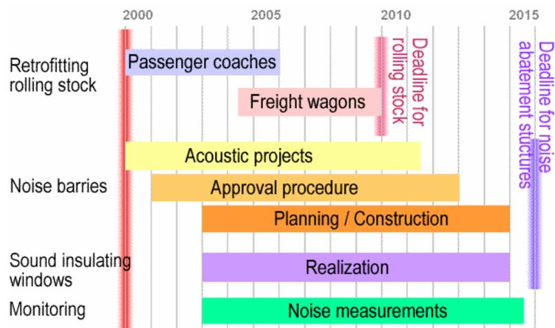
Fig. A-2: Time schedule of Swiss railway noise abatement plan. Noise barrier planning and implementation takes considerably longer than retrofitting wagons with composite brake blocks. This is because of the large number of individual projects.
